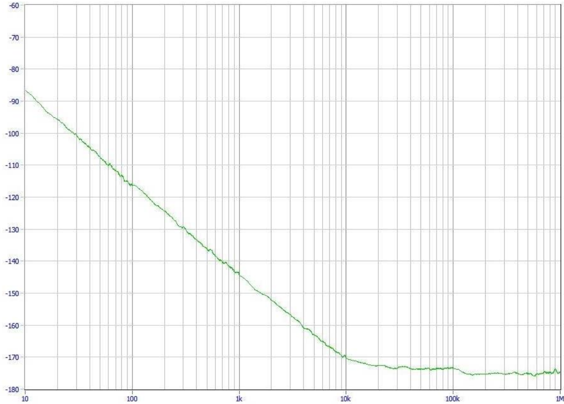
Typical Phase Noise at 100 MHz
